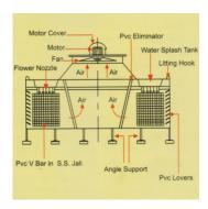
Induced draft cross flow principle for the operation. The tower design incorporates a frp distribution basin with no. Of flower type target nozzles in it and are located at the tower top. The water, by gravity, is dispersed over the fill media uniformly and water is allowed to pass Vertically down along the PVC V bar.
