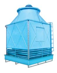
The Square Shape Cooling Towers Designed Especially For An Alternative To Round Model For Selection To Our Buyers. The Cooling Towers Consists Of Honey Comb PVC Fills And Eliminators In A Design That Maximizes Economy And Efficiency And Directly Driven Fan And Motor With Spray Nozzles With Minimum Drift Loss.
