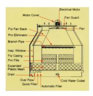
We Offer Cooling Tower In Rang Of 5 TR To 750 TR Capacities To Cool Water From 3 m³/hr To 450 m³/hr In Range Of 8 °C To 10 °C Temperature Difference & For More Than We Can Give In Multi Cell Cooling Tower In Any Range.
